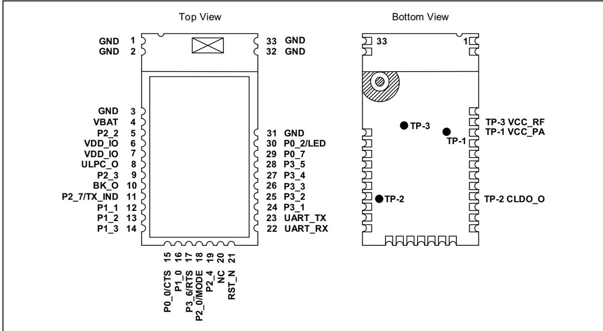
FIGURE 1-3: PIN DIAGRAM - RN4871U
