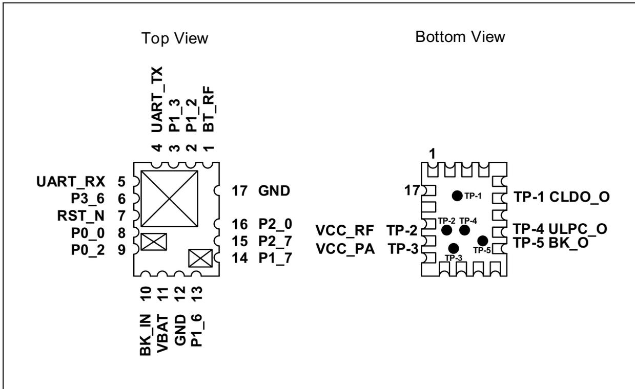
FIGURE 1-4: PIN DIAGRAM - RN4871
