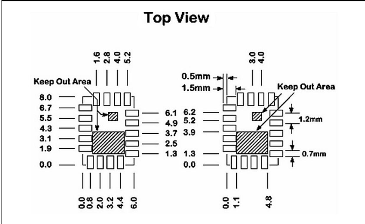
FIGURE 4-12: RN4871U RECOMMENDED PCB MOUNTING
