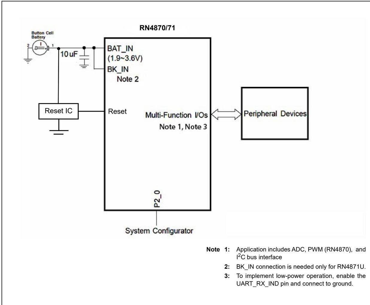
The Configuration pins on the RN4870 can also be configured through Windows<sup>®</sup>-based User Interface (UI) Configuration tool, BLEDK3.
