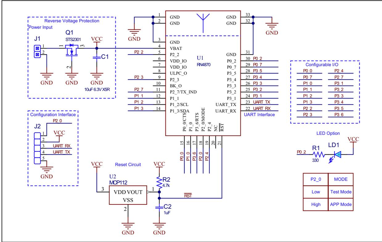
FIGURE 5-3: RN4870U REFERENCE CIRCUIT
